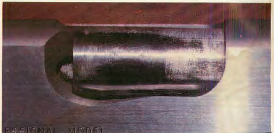
BELOW: Enlarged ejection port is worthwhile feature on weapon designed for self-defense.
